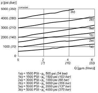
p = f(Q) Pressure - Flow rate characteristic  $[p_N = 5000 \text{ psi}]$
