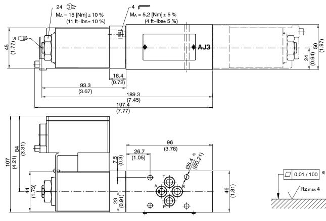
2/2 solenoid operated directional seat valve (single-solenoid model - solenoid A- or B-sided)
