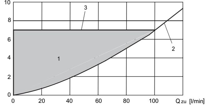
1 = Pressure loss area (The actual pressure-loss characteristic is dependent on the tank pressure at port B)
