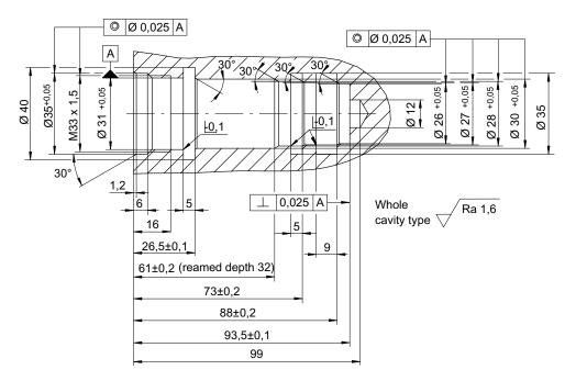
Form tool T2031 (order number: 100608916) to machine own cartridge cavities can be hired on request.
