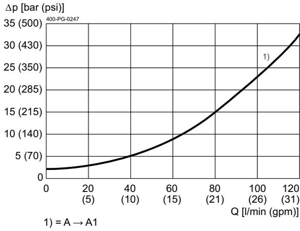
$\Delta p = f(Q)$  Pressure drop-flow rate characteristic
