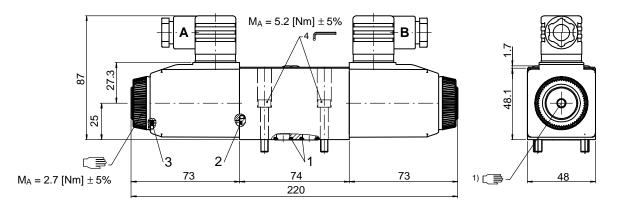
4/2 spool valve (1-solenoid model, A or B side)
