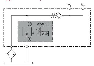
Manifold block with integral cooler-bypass thermostat valve
