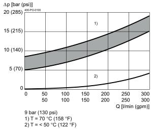
$\Delta p = f(Q)$  Pressure drop-flow rate characteristic
