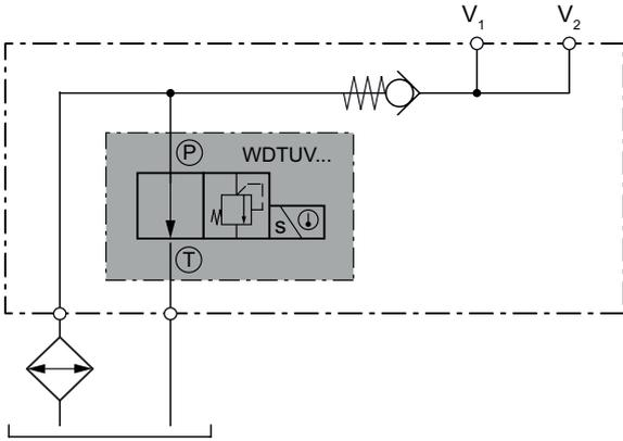
Manifold block with integral cooler-bypass thermostatic valve
