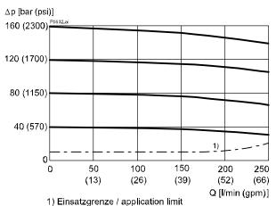
$\Delta p = f(Q)$  Pressure-drop characteristic (160 bar)
