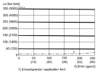
$\Delta p = f(Q)$  Pressure-drop characteristic (350 bar)
