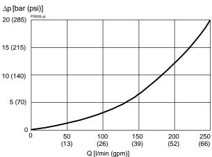
$\Delta p = f(Q)$  Pressure-drop - Flow rate characteristic (all pressure ranges)
