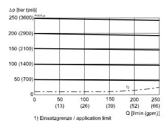
$\Delta p = f(Q)$  Pressure-drop characteristic (250 bar)
