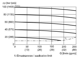
$\Delta p = f(Q)$  Pressure-drop characteristic (100 bar)
