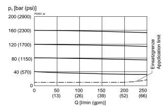
p = f (Q) Pressure - Flow rate characteristic  $(p_N = 40 \text{ bar})$
