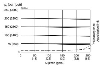
p = f(Q) Pressure - Flow rate characteristic  $(p_N = 100 \text{ bar})$
