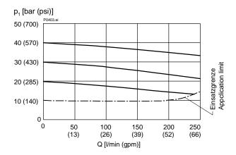
p = f(Q) Pressure - Flow rate characteristic  $(p_N = 250 \text{ bar})$
