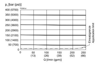
p = f(Q) Pressure - Flow rate characteristic  $(p_N = 160 \text{ bar})$
