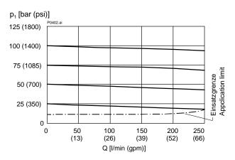
$\Delta p = f(Q)$  Pressure-drop - Flow rate characteristic (all pressure ranges)
