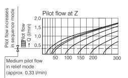
Rate of pressure change when turning the adjusting screw
