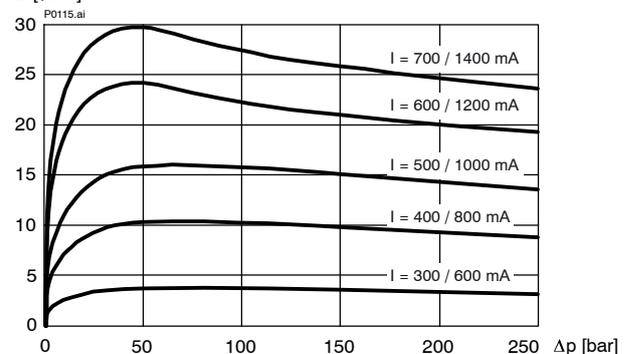
$Q = f(I; \Delta p)$  Flow rate adjustment characteristic [„120“]
