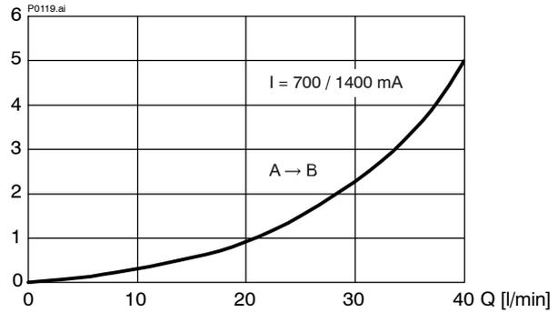
$Q = f(\Delta p; I)$  Flow rate adjustment characteristic [„300“]
