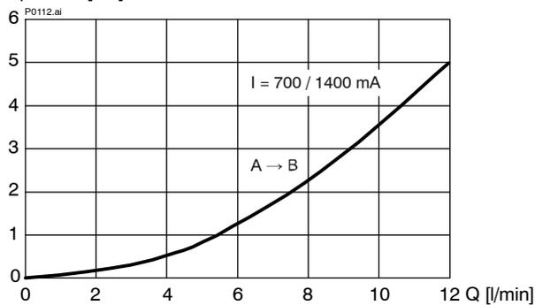
$\Delta p = f(Q)$  Pressure drop - Flow rate characteristic [„200“]
