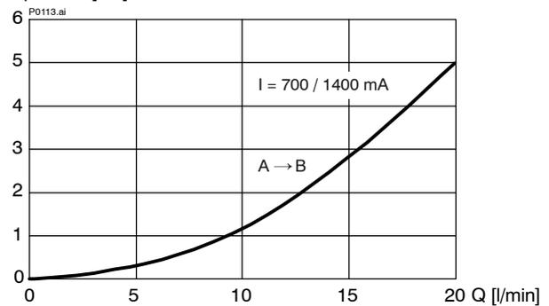
$Q = f(\Delta p; I)$  Flow rate adjustment characteristic [„120“]
