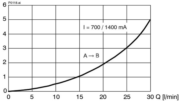
$\Delta p = f(Q)$  Pressure drop - Flow rate characteristic [„400“]
