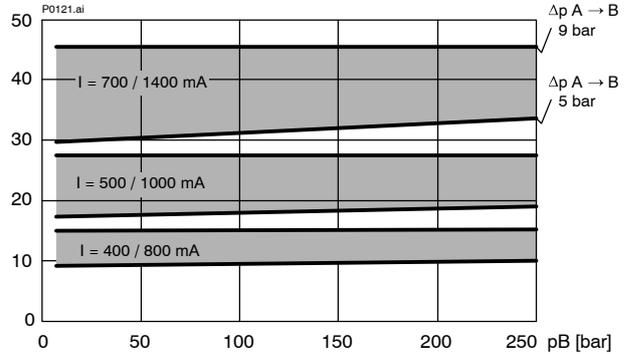
$Q = f(I; \Delta p)$  Flow rate adjustment characteristic [„300“]
