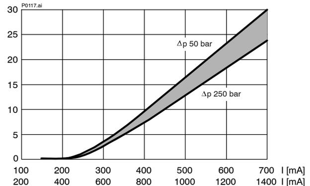
Must be used with pressure compensators -  $Q_N$  30 and 40 l/min
