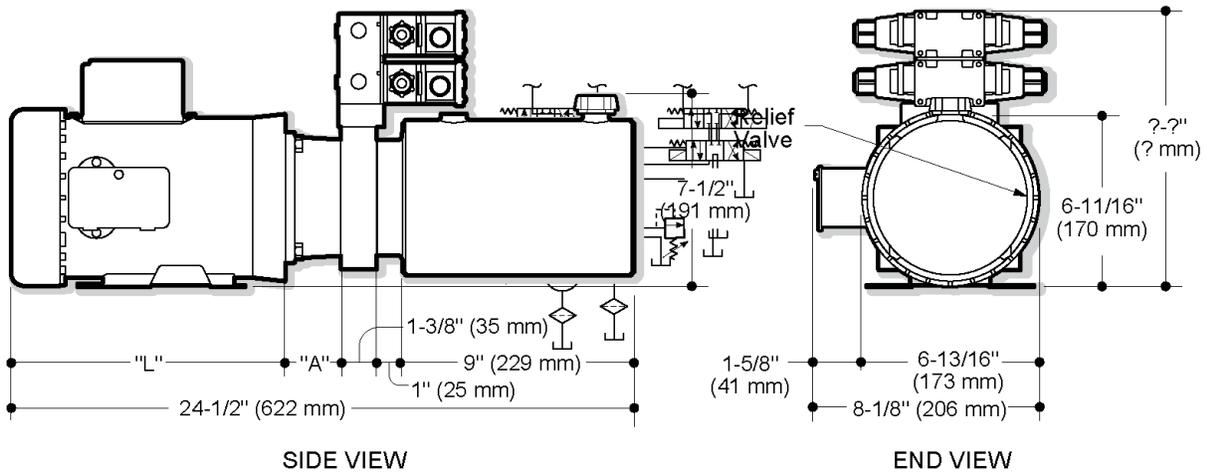
"L" dimension shown for 08751 motor is 10-11/16" (271 mm)
