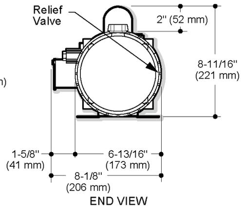
"L" dimension shown for 08751 motor is 10-11/16" (271 mm)
