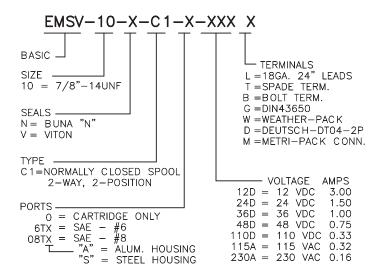
ALL L TYPE A.C. COILS ARE INTERNALLY A.C TO D.C. RECTIFIED. ALL S TYPE A.C. COILS USE A RECTIFIED DIN CONNECTOR
