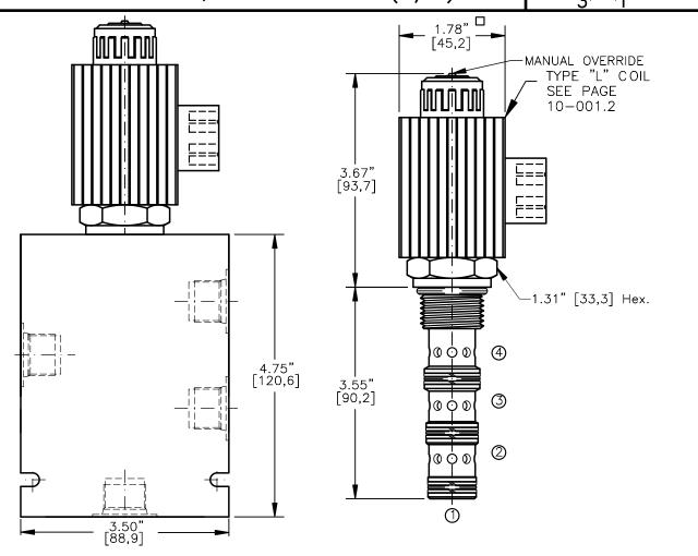
TORQUE: Steel = 70/75 Ft-Lb. [95/102 Nm] Aluminum = 55/60 Ft-Lb. [74/81 Nm]
