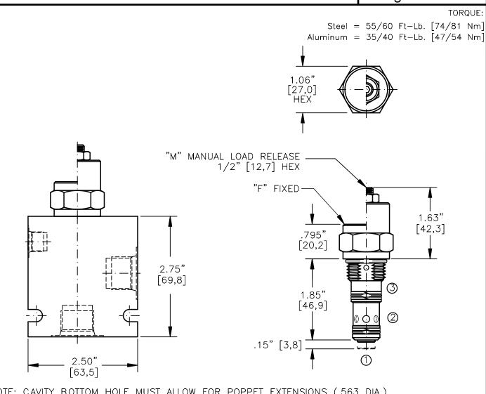
NOTE: CAVITY BOTTOM HOLE MUST ALLOW FOR POPPET EXTENSIONS (.563 DIA.) FOR ALUMINUM OR STEEL VALVE HOUSING CONFIGURATIONS SEE PAGE 0-022-1.
