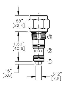
NOTE: CAVITY BOTTOM HOLE MUST ALLOW FOR POPPET EXTENSION (.500 DIA.). FOR ALUMINUM OR STEEL VALVE HOUSING CONFIGURATIONS SEE PAGE 0-021-1.
